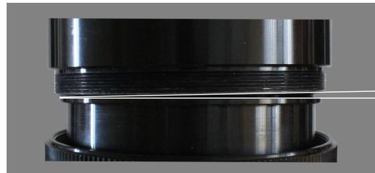
*Extension on focuser shows the mismatching of the bevel prevents flush connection*
