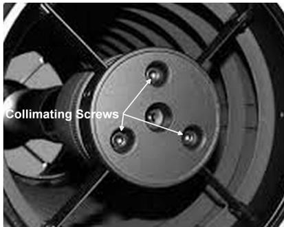
*Three Secondary Collimating Screws*
