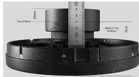
*The Measurement from the base to the top of the Secondary Mirror is 70.5mm which is 20mm below the top of the Baffle.*
